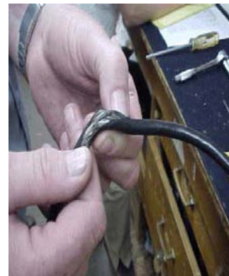
Fig. 4 Frayed cord exposing wires
